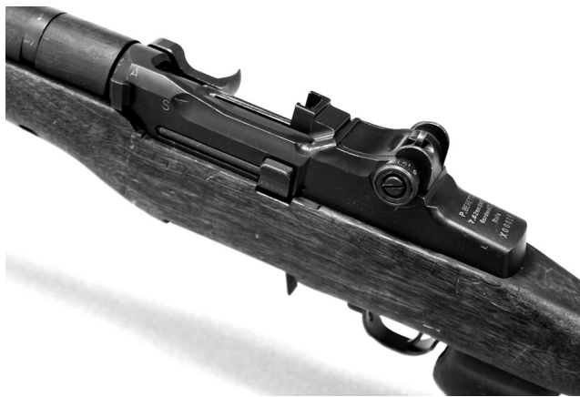
Figure 4.58 (See color insert.) Close-up of the BM59 receiver. Note the selector switch on the left side and the "P.B. BM59" marking on the action-lock button. The marking practices used by Beretta on the BM59 mimicked other manufacturers of the M14. Barely visible on the receiver below the sight-adjustment knob is the importer's mark "Springfield Armory," not to be mistaken for the government arsenal. (Image from author's collection.)
